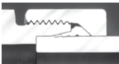
Two-edge cutting ring – deformation due to excessive tightening
